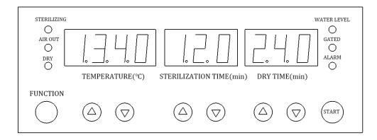
(1) **Function:** press this button for 5s can choose a function, press one time to display the A model (sterilization function); press again to B mode (sterilization, air release function); press again to display the A model, cycle like that.
