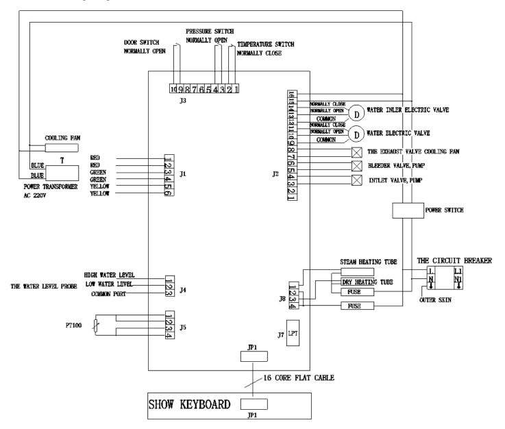
If necessary, we can provide circuit diagram and effecting the necessary information. If there is any doubt about electrical circuit repair, you can contact with our company.
